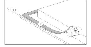
Stick the gasket (2) two millimeters from the external edge of the glass, after removing the protection sheet (3).
